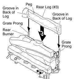
Figure 19 - Installing Rear Log (#3)
